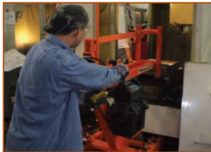
One of the many uses for Shop Lift™ is tool or mold loading in machine shops, especially when space is limited.
