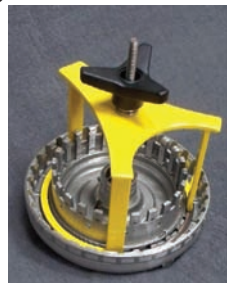
Recognize this drum? Nothing to fear as the “Z Buddy” is here. Note the ease of access to the snap ring. Also visible is the heavy duty ball bearing beneath the knob.
