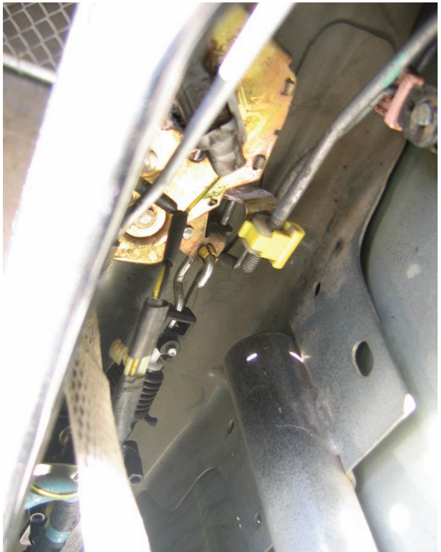
Figure 3: With the rear window track removed, you can get a good look at the driver's door latch assembly and power door lock actuator.
