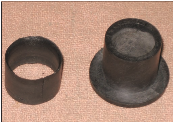
Figure 5: Compare worn bushing and new bushing
