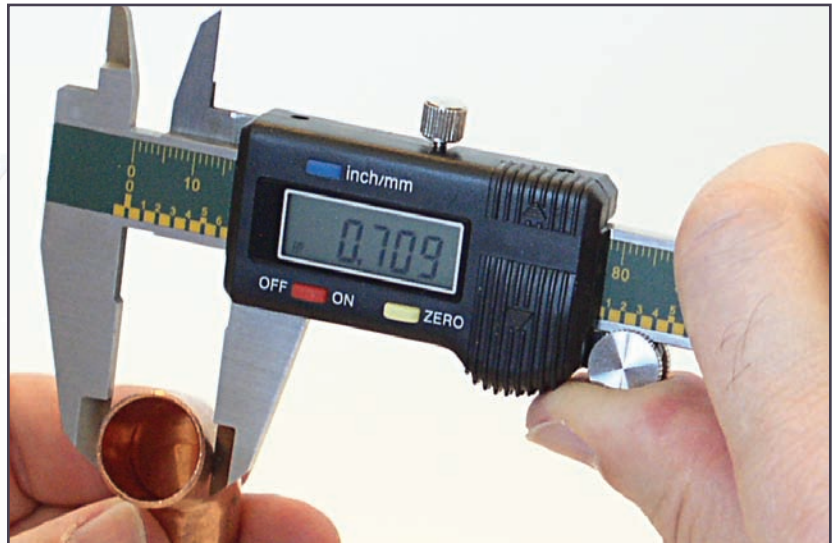
Figure 6: To measure the outer diameter of a component, apply the outside jaws gently around the widest part of the component. Not too tight! You don't want to crush anything, or screw up your measurement.
