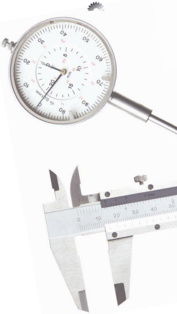
Figure 14: The ends of the fixed and moveable jaws align when the caliper is closed, so you can use the caliper to measure step height, too.
