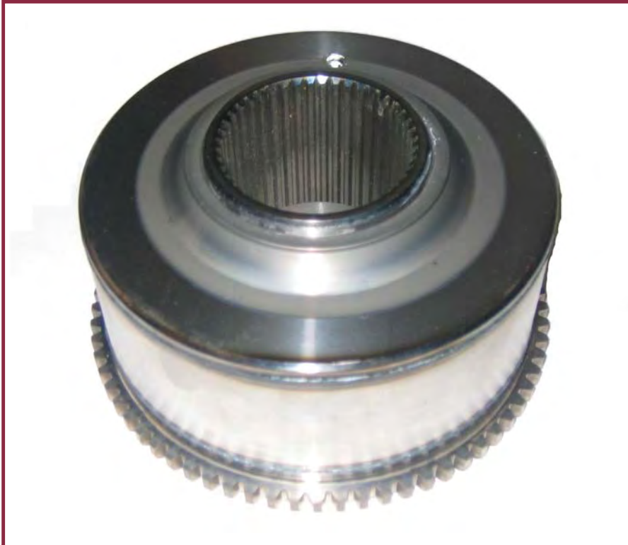
Figure 4: Totally enclosed viscous center hub driven by the mainshaft, the outer drives the chain cog. Inside is the same set of clutches, and the viscous coupler has a special fluid inside that allows it to keep full and provide a smooth slipping action of the clutches.
