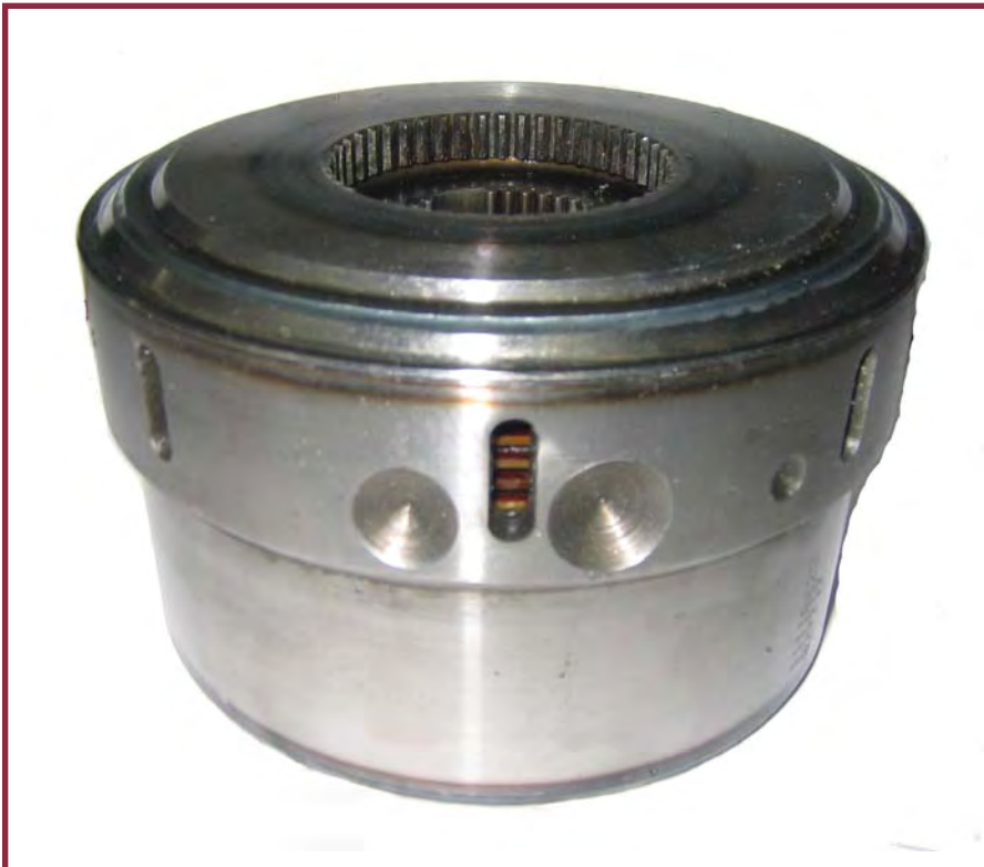
Figure 5: The inner splines are divided: one is driven by the mainshaft; the other drives a cog that drives the chain. This is an open viscous, as the slots indicate. This unit is called a progressive viscous. This viscous will slip less at one point because pressure will be added to stop it from slipping. And it produces an almost lock system as this occurs.
