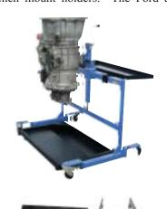
GM kit (430-FRD) comes with three brackets and inclusions to fit Ford E4OD, 4R100, C6, A4LD, 4R55E, AODE, AX4N and AXODE, as well as GM 350, 400, 4660, 4L80 and 4T60. An adapter is also available for the Allison 1000 and 2000 series. The Chrysler kit (430-CHR) comes as a three bracket set which will cover 413, 604, 670, 904, 500, 727, 618 and 606. Wherever possible, brackets have been made adjustable to fit multi-units.
