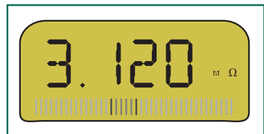
Figure 4: The "M" in front of the ohms symbol means "megohms," or ohms x 1,000,000. To determine the actual resistance, multiply the display by 1,000,000.
