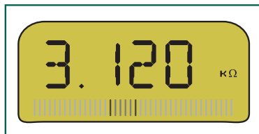
Figure 3: The "k" in front of the ohms symbol indicates that the meter is displaying "kilohms": ohms x 1000. You'll have to multiply the reading on the display by 1000 to determine the actual resistance.
